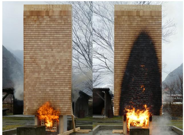
A fire test of the shingle facade
