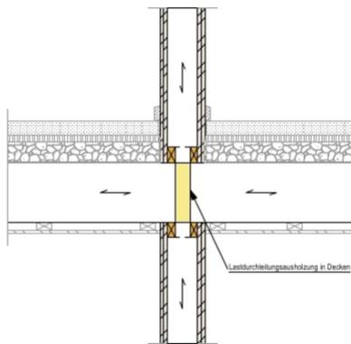
Detail load transmission apartment partition wall
