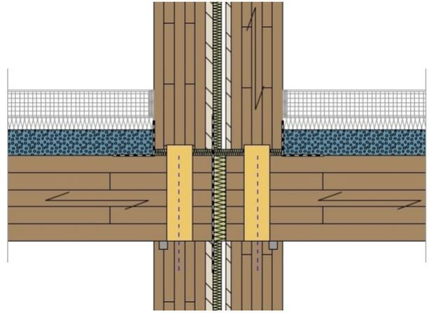
Load transmission detail with beech dowel
