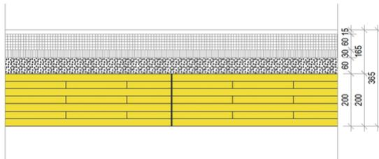
Ceilings made of CLT panels grouted with TS3 technology, with fill, impact sound insulation and underlay floor
