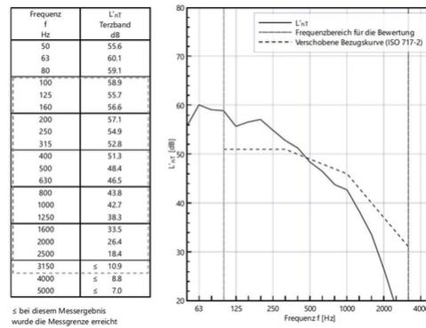
Impact sound measurements floor ceiling
