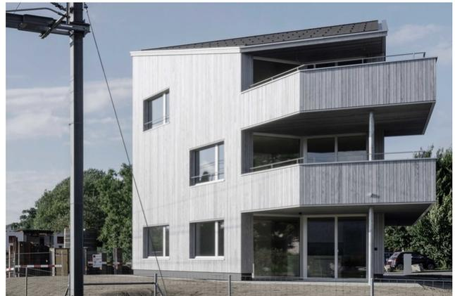
On Bachstrasse in Buchs in the canton of Aargau, a multi-family house was built in timber construction, which was originally planned as a reinforced concrete structure. The TS3 technology made it possible to change the material in the planning phase.
