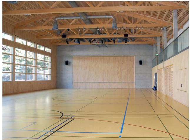
Sufficient space for the ventilation pipes thanks to the truss construction
