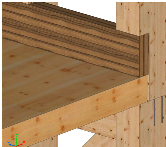
Visualization Cadwork - support on trusses
