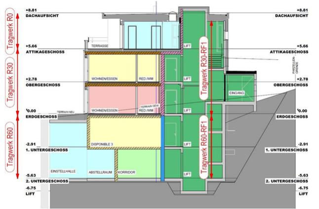
Section with the different fire sections
